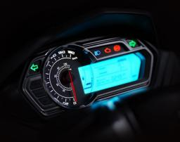
Automotive-grade Large LCD Instrument Panel Showing two sets of mileage memory, water temperature, total mileage, RPM, fuel, engine, ABS failure signal and all types of riding information clearly.
